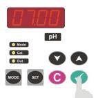
This time, the device shows 2.buffer solution value for a while and the device shows the electrode value which has not been calibrated yet again. At this time, electrode must be immersed in the 2.buffer solution.
