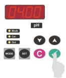
First buffer solution value is seen on the screen for a while and the device shows the electrode value which has not been calibrated yet. At this time, electrode must be immersed in the 1.buffer solution.
