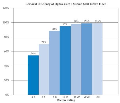
Cartridge micron rating is nominal. Data is representative of typical filter performance using SEA test dust.
