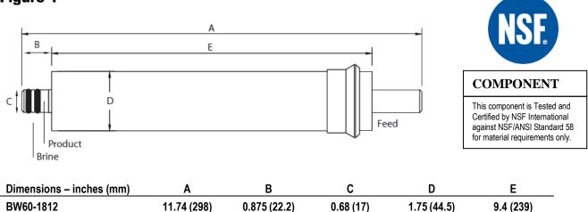
1. BW60-1812 Home Drinking Water elements seal at a standard 2.0 inch – 2.05 inch I.D. within pressure vessels
